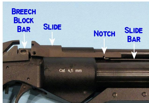
Step 3: The slide is under spring tension, and you can lock it out of the way by moving it forward until you can swing the slide bar (#7) to the right to catch in a notch in the slide. (see photo, above right)
