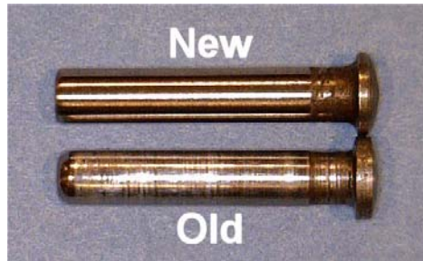
Figure 3: New & old valve designs
