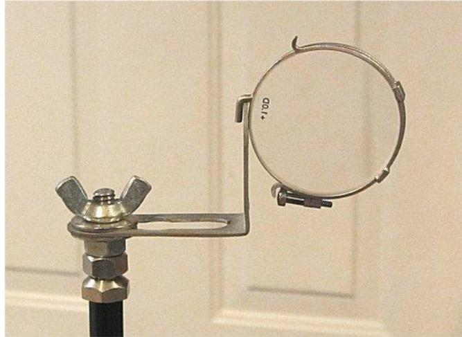
Once the light is set up, you can hold the lens and move it until you get a small focused spot on the white door. If you set up the stand to hold the lens a little bit closer to the light, you can leave that in a fixed location, and move a white piece of paper back & forth to get a more precise distance for  $\tilde{o}$ .
